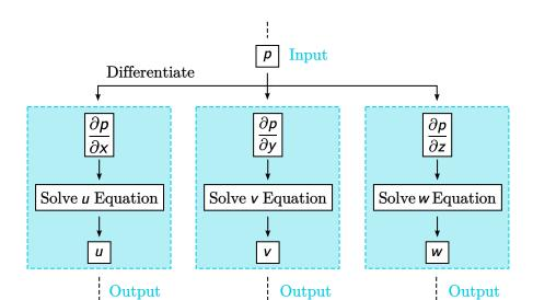
For the pressure gradients  $\partial p/\partial x$ ,  $\partial p/\partial y$  and  $\partial p/\partial z$  to be consistent, it is easier to start with an input pressure field p and use numerical differentiation (covered in a future lecture) to calculate the pressure gradients in each direction.
