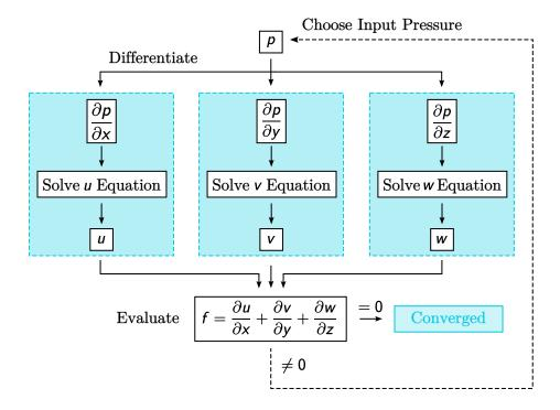
The central idea in the conceptual algorithm (and the SIMPLE algorithm) is to keep choosing different input pressure fields until the computed velocity field satisfies both the continuity and Navier-Stokes equations (resulting in f = 0).
