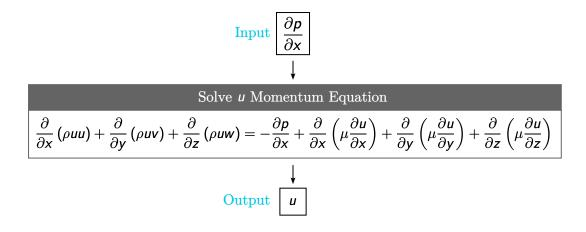
1. Choose an input pressure gradient,  $\partial p/\partial x$
