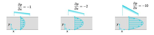
It follows that different pressure gradients result in different velocity profiles. We are going to use this idea to develop the central idea of the conceptual algorithm. Applying different pressure gradients results in different velocity profiles.
